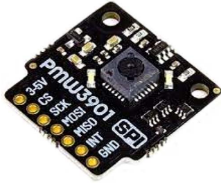
Figure 4. The Pimoroni PMW3901 optical flow sensor.
