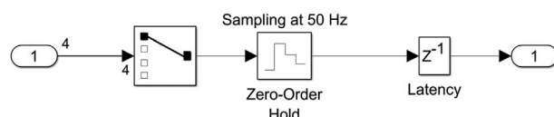
Figure 14. Inertial measurement unit Simulink block diagram.
