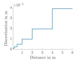
Fig. 7. Discretization of depth values, i.e., the distance between a value and the next possible one, depending on the distance.
