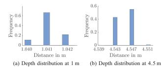
Fig. 9. Representative probability distributions for nonfringe depths values at different distances. The gaps between values are due to the discretization. (a) Depth distribution at 1 m. (b) Depth distribution at 4.5 m.
