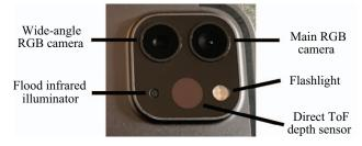
Fig. 3. Sensors on the back of the iPad Pro 2021. Width and height of the panel are around 27 mm.
