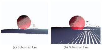
Fig. 17. Point cloud of the plastic sphere being observed by the iPad depth sensor. Best-fitting sphere overlaid in red. Floor appears wider at 2 m due to the field of view. (a) Sphere at 1 m. (b) Sphere at 2 m.
