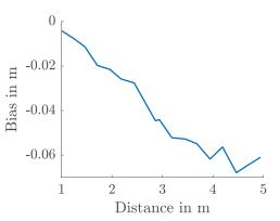
Fig. 8. Difference between the ground truth depths and the measured depths at difference distances. The negative bias means that the measured values are smaller than the ground truth.
