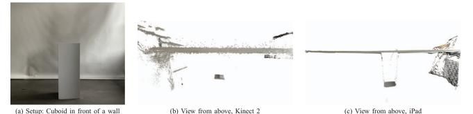
Fig. 11. Setup of the cuboid in front of wall, observed by a Kinect 2 and an iPad positioned next to each other. Note how the Kinect 2 produces spatially uncorrelated noise, while the iPad produces a smooth, almost flat surface that shifts and deforms each frame. (a) Setup: cuboid in front of a wall. (b) View from above, Kinect 2. (c) View from above, iPad.
