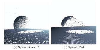
Fig. 15. Plastic sphere of radius 15 cm lying on the ground, being observed from a distance of 2 m by a Kinect 2 and an iPad depth sensor. (a) Sphere, Kinect 2. (b) Sphere, iPad.
