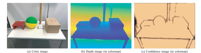
Fig. 2. Example capture of the scene from Fig. 1 showing the three video streams of the iPad depth system: the color image (1920 × 1440 px, RGB), the depth image (256 × 192 px, 32-bit float array), and the confidence image with 256 × 192 pixels, 1 byte/px, and three possible discrete values: low (black), middle (brown), and high (orange) confidence. (a) Color image. (b) Depth image (in colormap). (c) Confidence image (in colormap).
