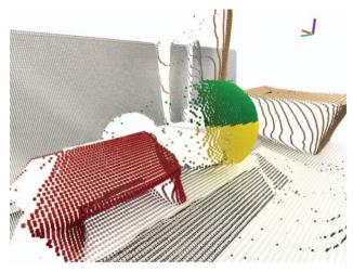
Fig. 1. Example of reconstructed point cloud for a table scene with objects, captured by an iPad Pro 2021 tablet.
