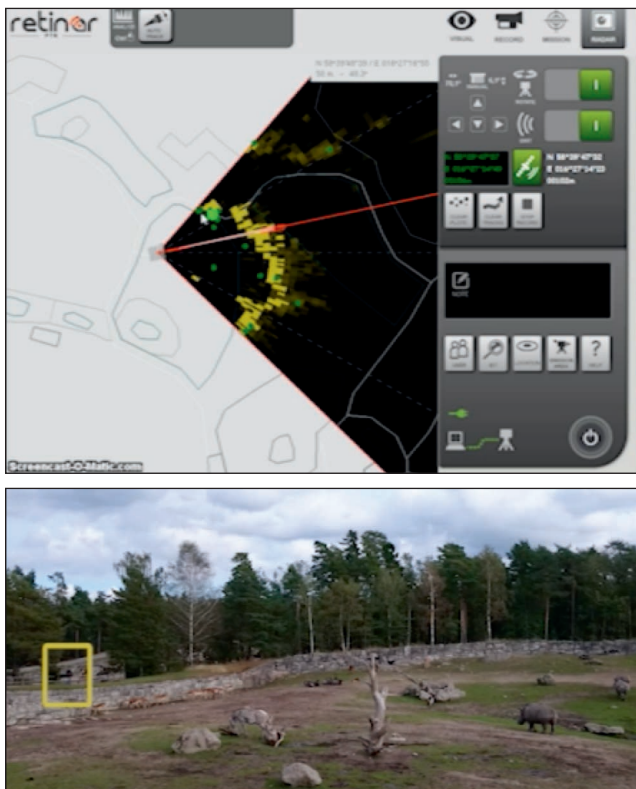
Figure 4 The top picture shows the operator view of a radar system, where the green dots mark the detections. The right view shows an image from a camera mounted on top of the radar. There is a rhino to the right and a human marked with yellow to the left. Top picture provided by Meteksan Savunma.
