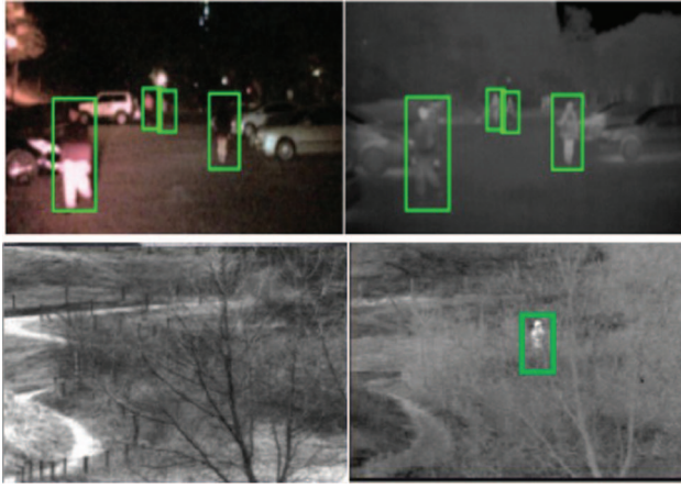
Fig. 1. Two different scenarios of visual context of actions captured by two different sensors: low-light VIS and IR sensors. Each sensor has its limitation that affects recognition performance. It means contextual improvement can play a positive role in improvement of detection capability of autonomous systems.
