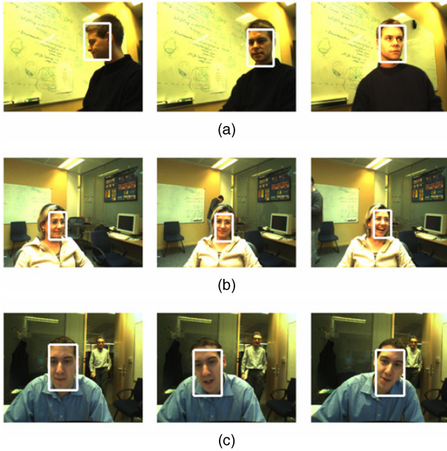
Fig. 28. Examples of face localization by our system on videos with the number of faces correctly localized. (a) Jamie sequence: 40 correct localization/43 images. (b) Ilkay sequence: 72 correct localization/80 images. (c) Geoff sequence: 24 correct localization/24 images.
