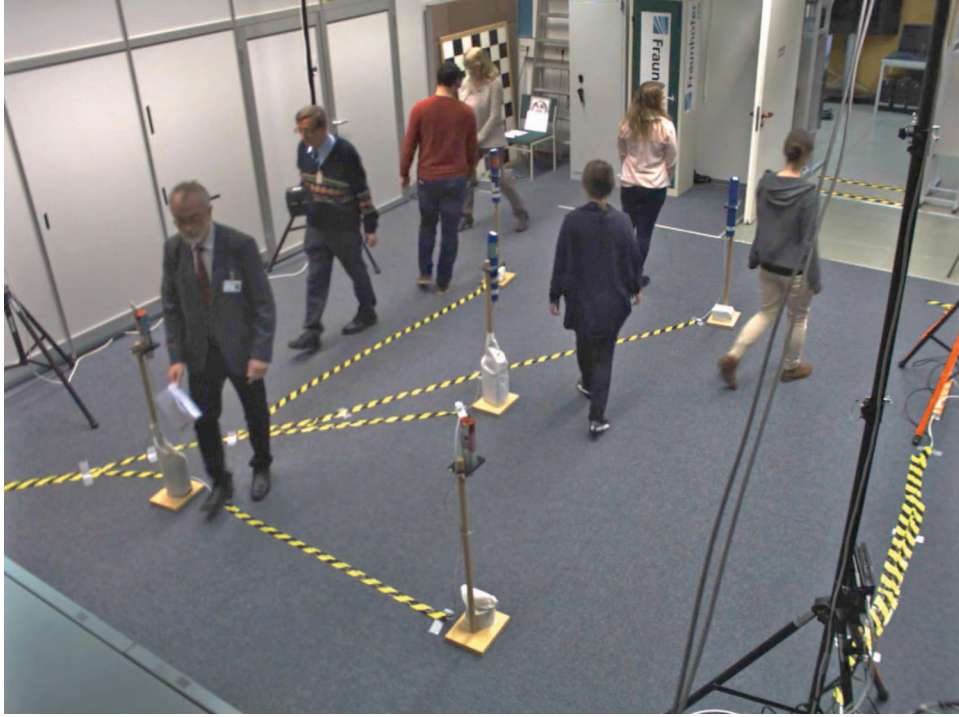
Fig. 6. Lab view of demonstrating IRDD localization in person streams using five gamma sensors on stabs and ToF cameras at the ceiling (invisible).
